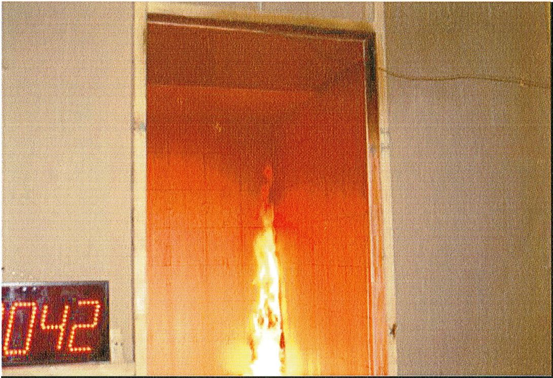
Figure B-3. View of Burner Corner; 42 s into Test.
