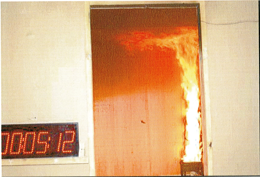
Figure B-5. View of Back Wall; Burner Increased to 160 kW; 5 min 12 s into Test.
