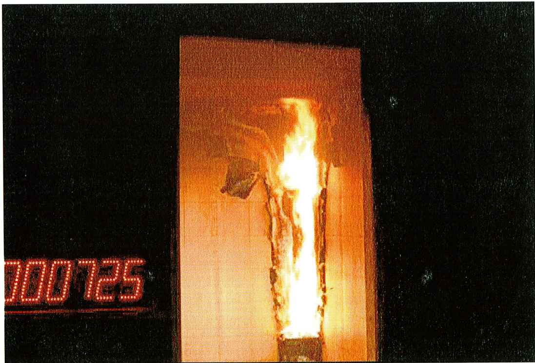
Figure B-6. View of Burner Corner; 7 min 25 s into Test.
