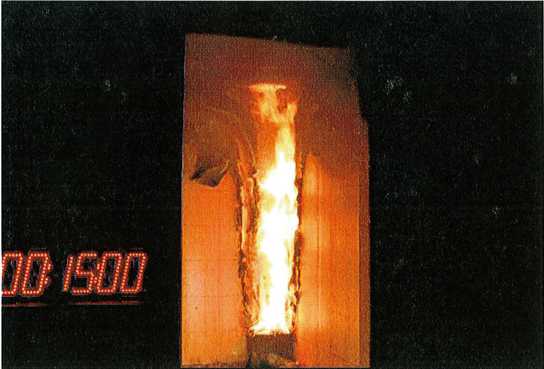
Figure B-7. View of Burner Corner; 15 min into Test; Test Complete.
